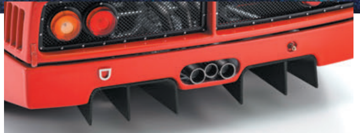
The muffler used the same three pipes as the F40 with the center exhaust as the wastegate for controlling the turbo pressure.
