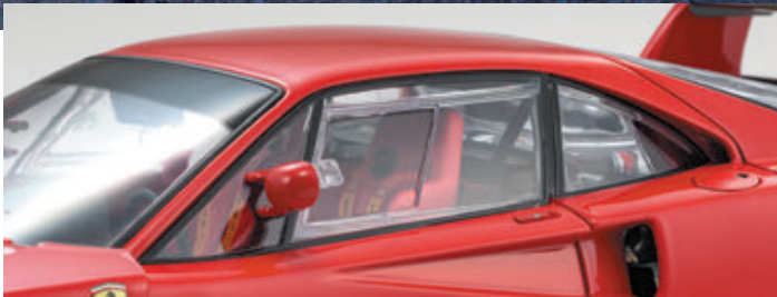
Designed for motorsports, the Competizione features acrylic side windows with a sliding function instead of a typical lifting mechanism to reduce weight.
